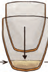
5. Insert small pot in large pot and add sand to outside of small pot
