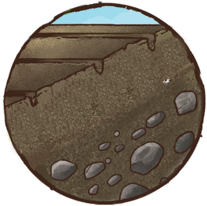
4. Improved practice: use stick to create shallow trenches perpendicular to slope
